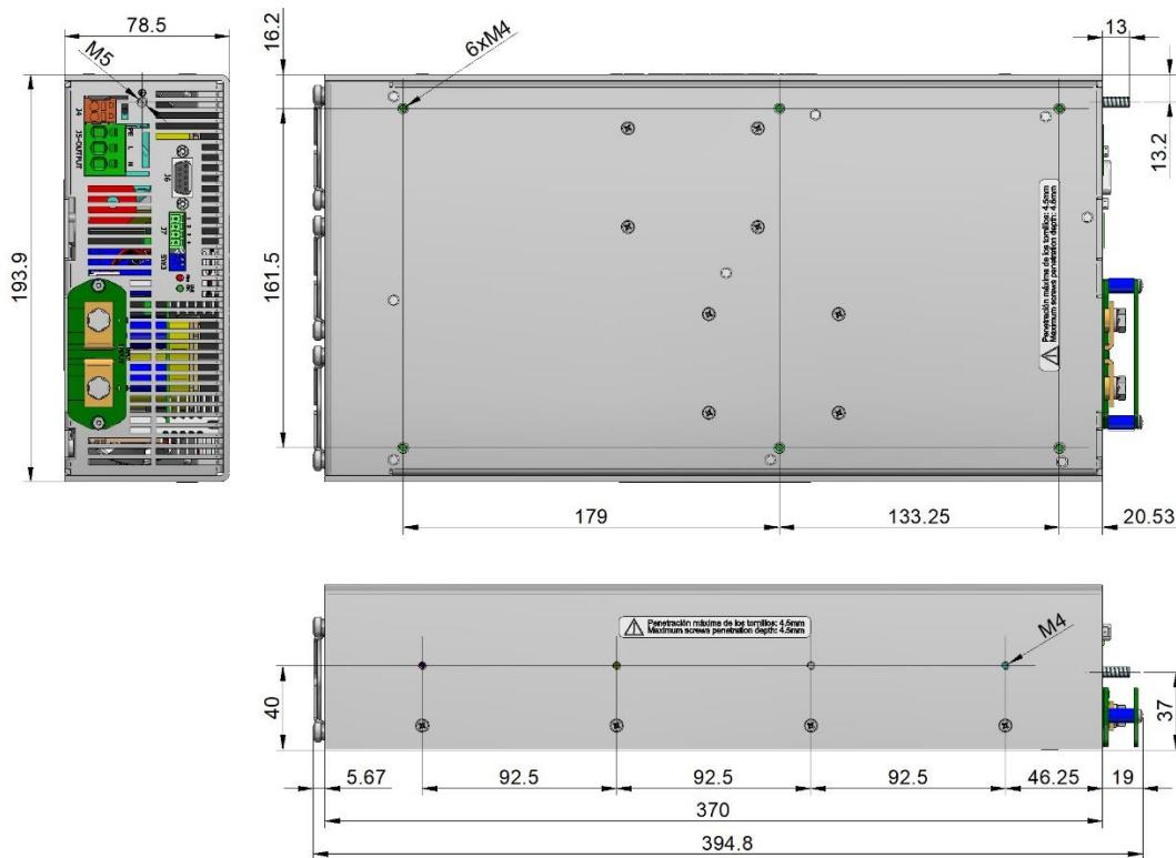
Maximum depth for the screws M4: 4.5mm
