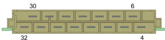
CONECTOR / CONNECTOR DIN 41612 H15 - Max. 12A / Terminal
